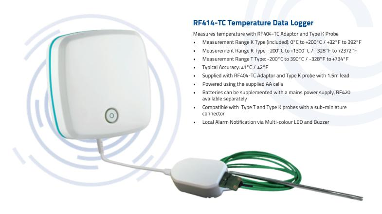
**Note:** The RF414-TC is supplied with the RF404-TC adaptor and probe unit. The adaptor can be used for a range of Type T or Type K probes manufactured by Comark Instruments. The RF414-TC data logger can be used as dual channel but an additional RF404-TC adaptor will need to be purchased.
