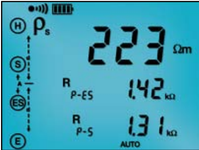
The Schlumberger test displays test lead connection, soil resistivity ( \rho ) test results, test electrode resistance and more.
