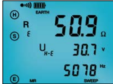
The 3-Point Fall-of-Potential test displaying test lead connection, grounding electrode resistance, test voltage and frequency.
