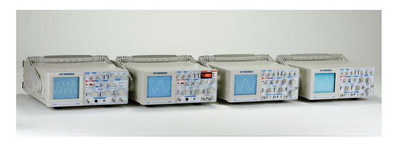
B&K Precision's 212x Series are dual trace oscilloscopes that offers high performance at a low price. Most competitor's entry level oscilloscopes have a 20 MHz bandwidth, while B&K Precision's 212x Series have a bandwidth of 30-60 MHz.
