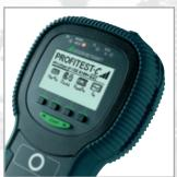
Test Instrument for IEC 364-6
