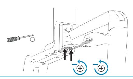
2 Loosen or tighten this bolt to adjust tilt to desired angle.
