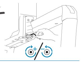
3 After desired tilt is achieved, retighten these two screws to secure.
