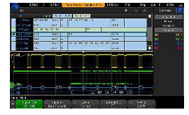
Figure 19: Multi-bus time aligned decode
