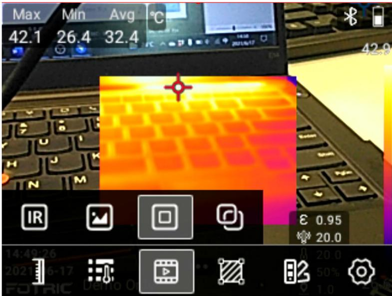
By default, the thermal display area is 1/4 of the entire screen. Users can adjust the thermal image areas and position by touch-screen, as the below following images:
