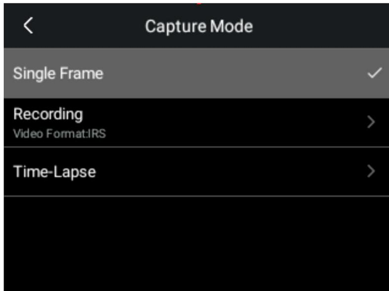
The device can be set to take single frame picture, record IRS radiometric /MP4 videos or time-lapse pictures.
