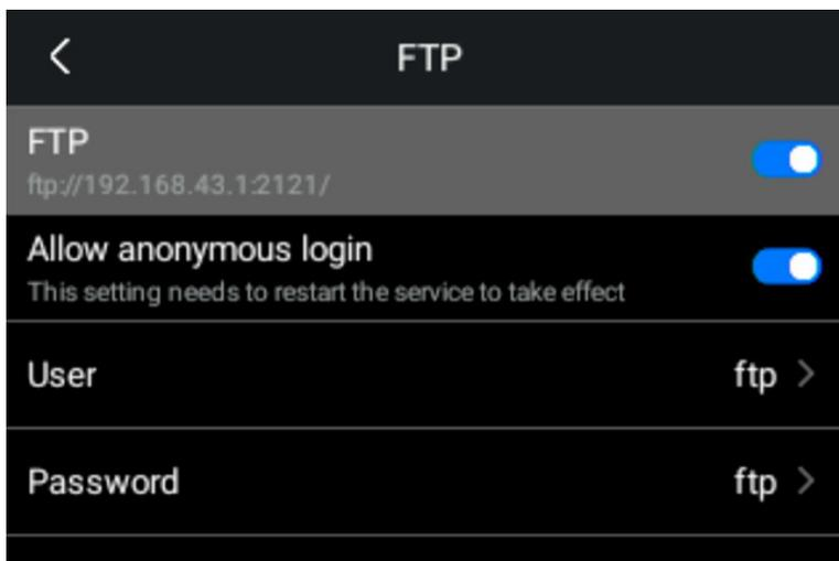
When the FTP Transfer function is turned on, the thermal camera's storage data (TF card) can be transferred to a computer via FTP protocols.
