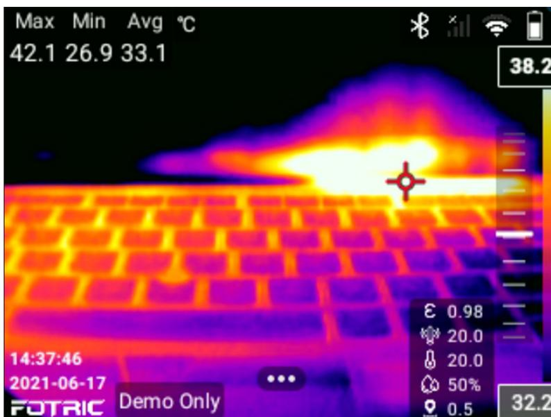
As shown in the image below, the upper and lower limits are selected. And the range of temperature scale can be adjusted by up and down direction key
