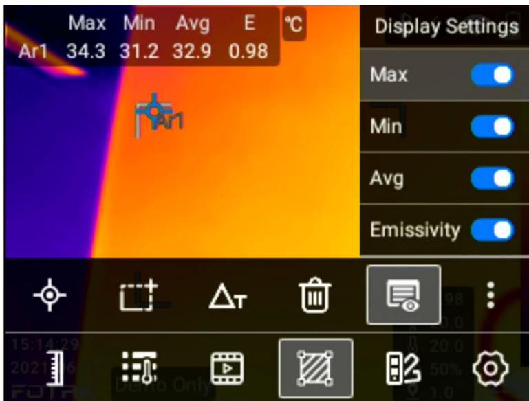
The available options for display are maximum, minimum, average temperature and emissivity. The default display is the maximum temperature.
