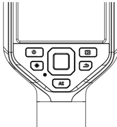
To turn on the thermal imager, long-press the Power Button
