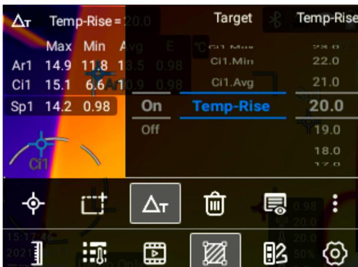
The 'Temperature difference' feature is available through touch-screen and press-button. If you need to activate 'Temperature difference', please perform the following procedures:
