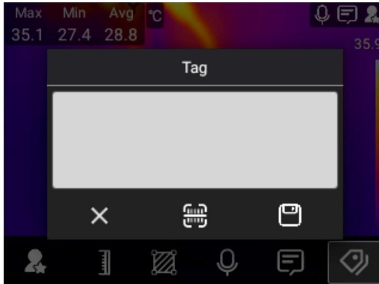
In the image freeze interface, Tag information can be inputted by QR code scanning and virtual keyboard
