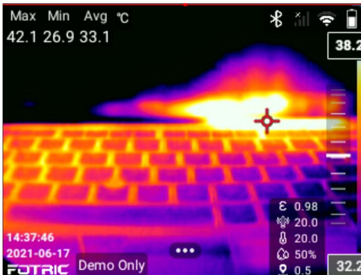
As shown in the figure below, the upper limit of the temperature scale can be adjusted separately by using the slider:
