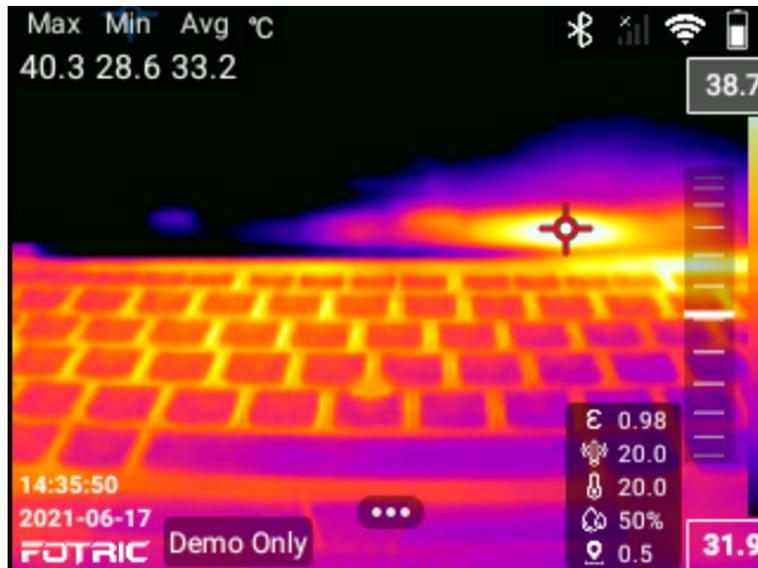
As shown in the figure below, both upper and lower limits of the temperature scale are locked and cannot be adjusted:
