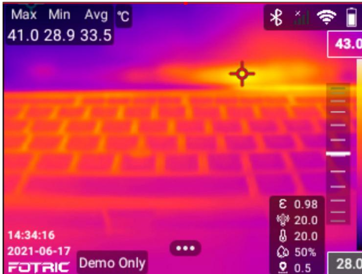
As shown in the figure below, the lower limit of the temperature scale can be adjusted separately by using the slider
