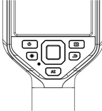
The AI programmable key can call upon different functions according to the user's need. It is available on the main interface, image freeze interface, and gallery's image analysis interface.
