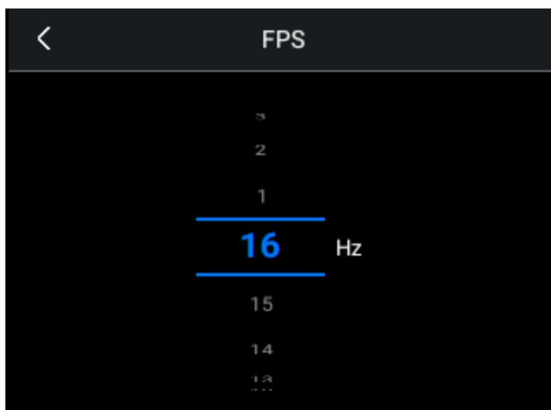
1. In video recording mode support FPS(1~16Hz) full-radiometric thermal video recording.
