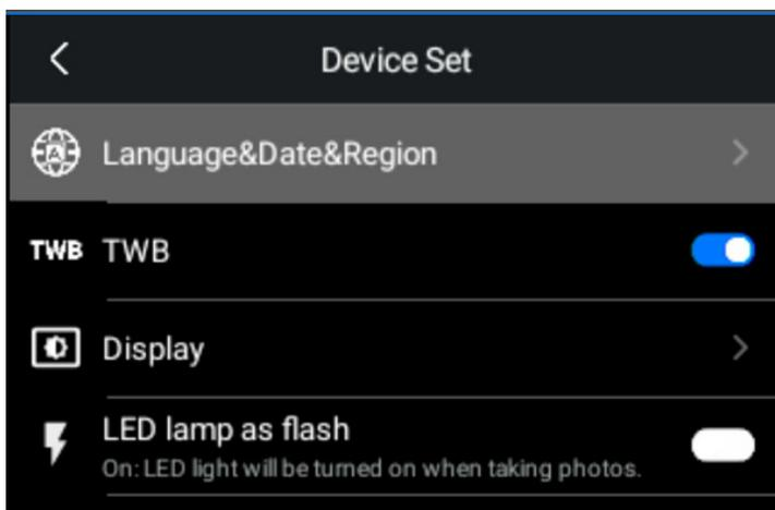
TWB mode: TWB is named Thermal White Balance. It balances color distribution on the entire temperature span of the image.
