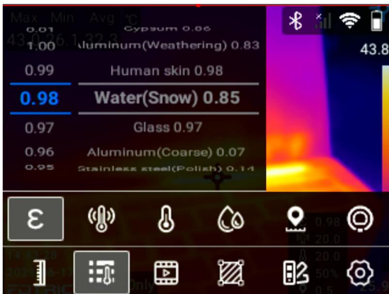
**ε** The emissivity settings of the FOTRIC thermal imager have 2 options: Fullscreen emissivity correction and partial emissivity correction.
