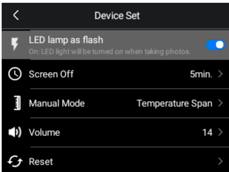
The LED lamp on the thermal imager can serve as a flash for the digital camera. When this function is turned on, the thermal imager will activate an LED flash lamp when capturing images. The LED can also be turned on permanently on the Swipe-down menu.
