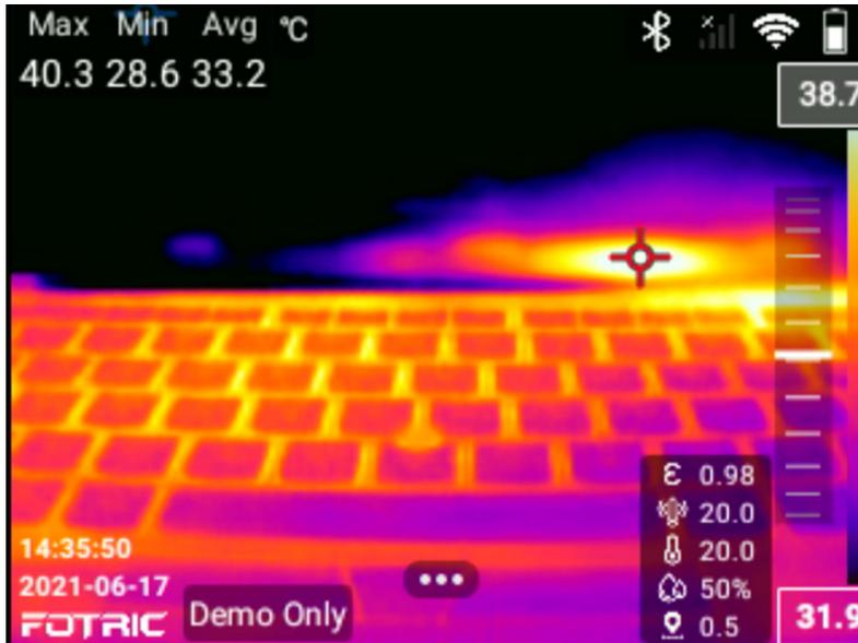
As shown in the image below, the lower limit is selected. And the lower limit of the temperature scale can be adjusted by up and down direction key
