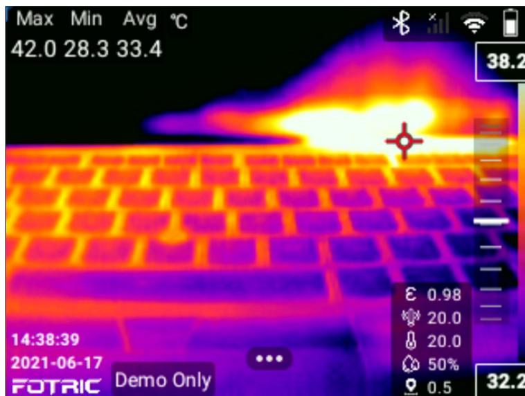
Users can adjust the upper or lower limit by pressing the left and right direction keys. The selected limit is displayed in gray.
