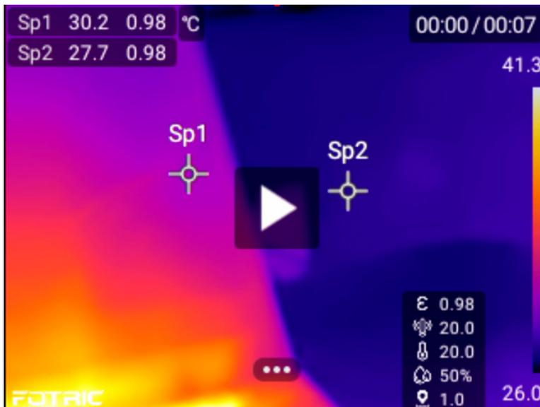
Users can preview the radiometric image before saving it. On the freeze interface, videos can be analyzed. Pressing the trigger button again to save the video.
