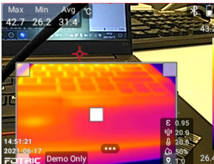
3. When specific ROI is selected, 'Resize' and 'reposition' mode can alternate by pressing the 'OK' button. Pressing the 'Return' button can exit editing mode.
