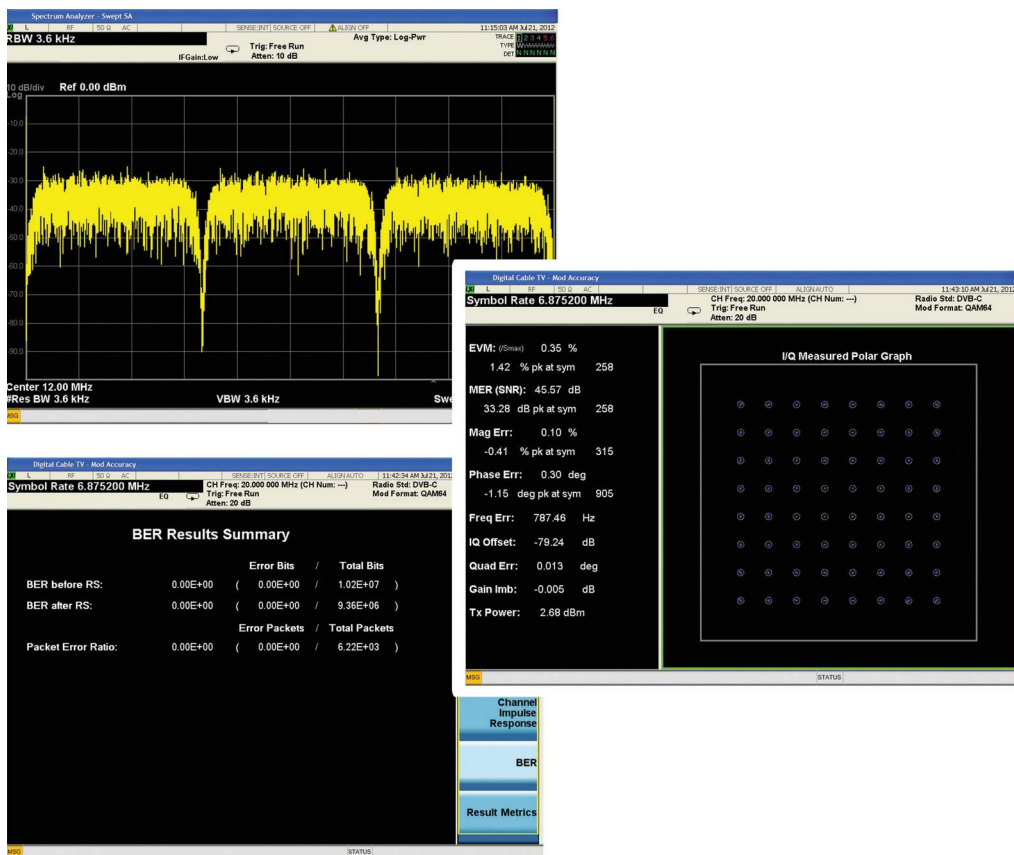
Figure 11. Three DVB-C 64QAM carriers generated simultaneously by a Keysight 33522B. Tests are performed in the central channel, but all are channel coded following the DVB-C standard—although the data is uncorrelated to avoid artificially high power peaks in the combined signal. The DVB-C analysis shows the modulation quality obtained (EVM = 0.35%). Since the signal is properly channel coded, it is possible to perform BER tests with it. BER can be calculated by checking the corrected and uncorrected errors before and after Reed-Solomon decoding.
