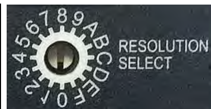
Point the notch in the switch stem to assign the rotary position.
