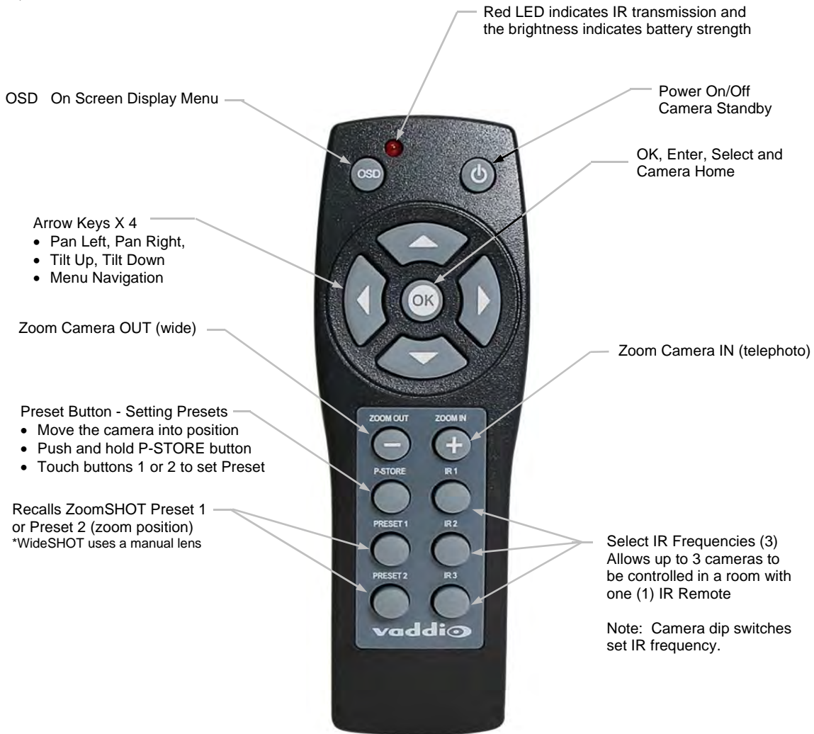
Image: Vaddio IR SHOT Commander Hand-held IR Remote (Top View)
