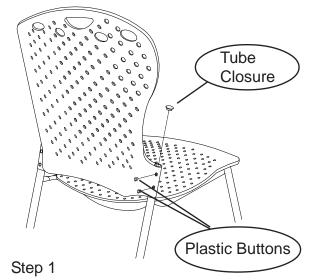
Remove the large plastic tube closure and the two plastic buttons that hold the right side back on your chair.
