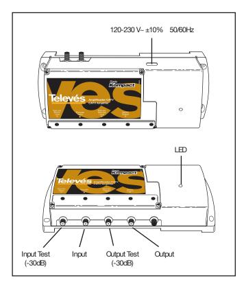
This product has been manufactured in a fully shielded zamak enclosure and the gain can be selected on site.
