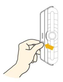
Slide the eBeam Edge into the Edge Battery Pack as shown until you feel the battery pack snap into place.
