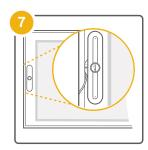
Place the receiver so that it is centered vertically on the board, and parallel to the frame.
