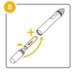
Locate the eBeam stylus and twist open the battery cartridge. Install AAA battery in your eBeam stylus.
