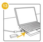
Connect the wireless adapter to the USB port.
