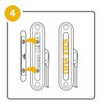
Place a mounting plate onto the back of the receiver with the Command adhesive side facing out.
