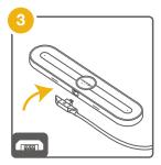
Connect the eBeam USB cable to your eBeam receiver.
