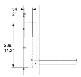
Integrated laptop shelve, can be closed with a padlock in up position (padlock not included) for mini computer or laptop.
