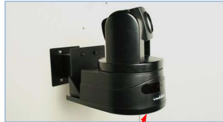
Fig. 13: CONCEAL Lower Cover Plate locked in place
