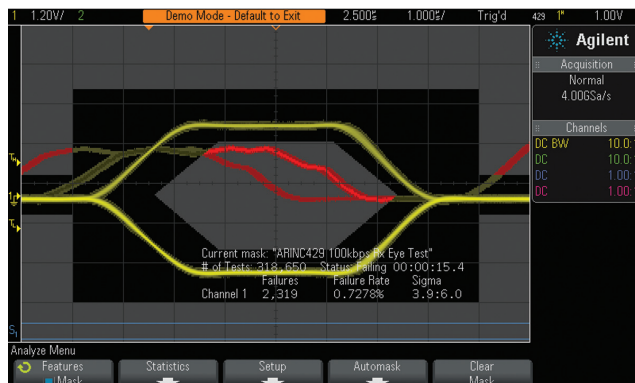
Figure 2: Testing the signal integrity of a differential ARINC 429 serial bus using eye-diagram mask testing.
