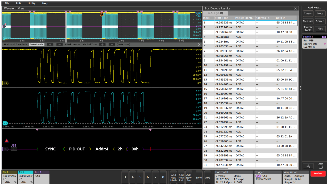
Figure 23: Triggering on a USB full-speed serial bus. A bus waveform provides time-correlated decoded packet content including Start, Sync, PID, Address, End Point, CRC, Data values, and Stop, while the bus decode table presents all packet content from the entire acquisition.
