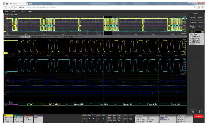
Figure 33: e*Scope provides simple remote viewing and control using common web browsers.
