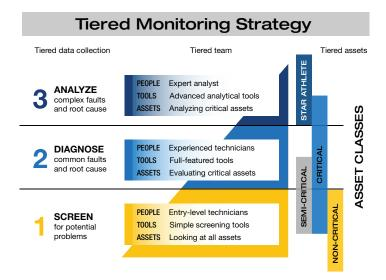
Screening, diagnosing, and analyzing are all forms of vibration monitoring. Vibration screening offers the greatest initial value by providing a simple scalable solution to extend asset coverage, reduce routes and minimize labor costs.
