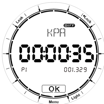
Figure 8 Pressure leak test finish interface
