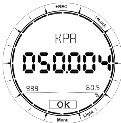
Figure 10 pressure record operation interface
