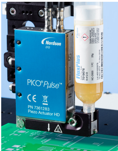
PICO Pulse® jetting FluxPlus onto a PCB.
