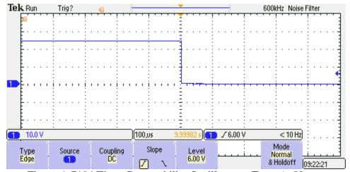
Figure 6: 7194 Timer Repeatability Oscilloscope Trace (± 50µsec
