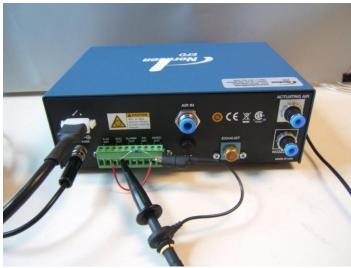
Figure 1: Timer Accuracy Oscilloscope Connection
