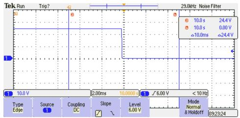
Figure 5: 7194 Timer Accuracy Oscilloscope Trace (± 5 msec)
