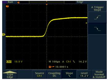
Figure 3: Timer Repeatability Oscilloscope Trace (± 50µsec
