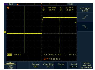
Figure 2: Timer Accuracy Oscilloscope Trace (± 5 msec)
