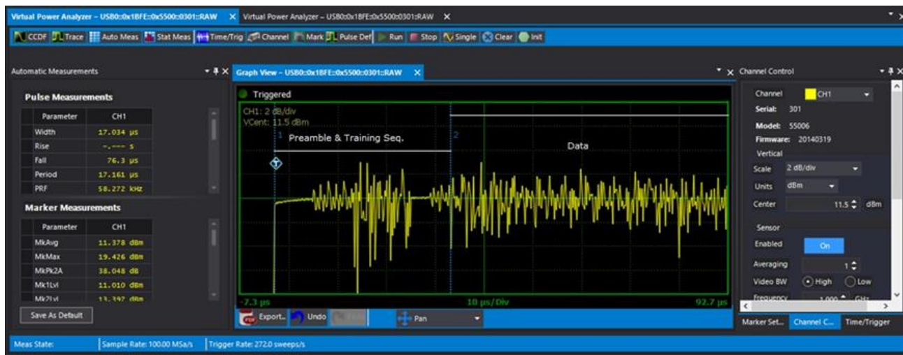
Fig.1: Preamble, training sequence and data burst of the WiFi signal
