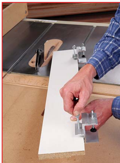
Patented Swing Arm design allows you to accurately rip wide boards with ease
