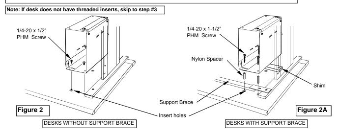
A. Determine whether the CPU Sling will mount on the right or left side of the desk and align the top sling holes with the appropriate set of inserts. Figure 2 shows a sling being mounted on the left side of a desk.
