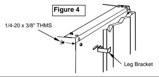
Note: If the CPU Sling is being used on a CLASS™ or Evolution™ desk, the included (042019) Leg Bracket should be attached to the Sling and Front Leg.
