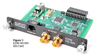
Using only the most advanced and leading edge 3Gb/s single link HD-SDI components available today, the EZIM HD-SDI Slot Card produces remarkable picture quality with video resolutions of up to 1080p/60Hz over a single coax cable. The EZIM HD-SDI Slot Card also features a 36VDC RJ-45 EZCamera connector for powering HD-18 up to a distance of 500' (152.4m) when using the Vaddio Quick-Connect CCU controller.
