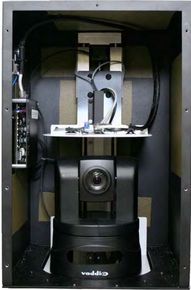
Figure 15: Vaddio ClearVIEW HD-18 PTZ HD Camera mounted on the Camera Lift Platform
