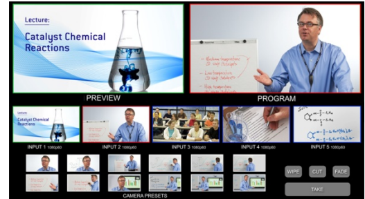
TeleTouch Touch Screen Control Panel with Multi-View Five-Input Layout
