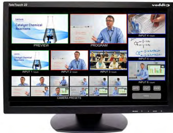
TeleTouch 22" HD Touch Screen LCD Monitor with Base (Simulated ProductionVIEW Multiviewer Output)
