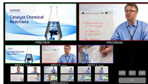
TeleTouch Touch Screen Control Panel with Multi-View Four-Input Layout Three-Inputs Displayed
