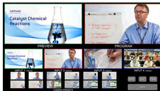
TeleTouch Touch Screen Control Panel with Multi-View Four-Input Layout
