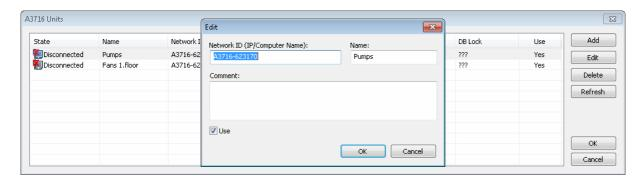
Push the A3716 Units button. Select the A 3716 unit. Push Edit button. Uncheck the Use box and push OK. All readings made by this unit will be stopped. When you check back the Use box then the readings will be taken again.
