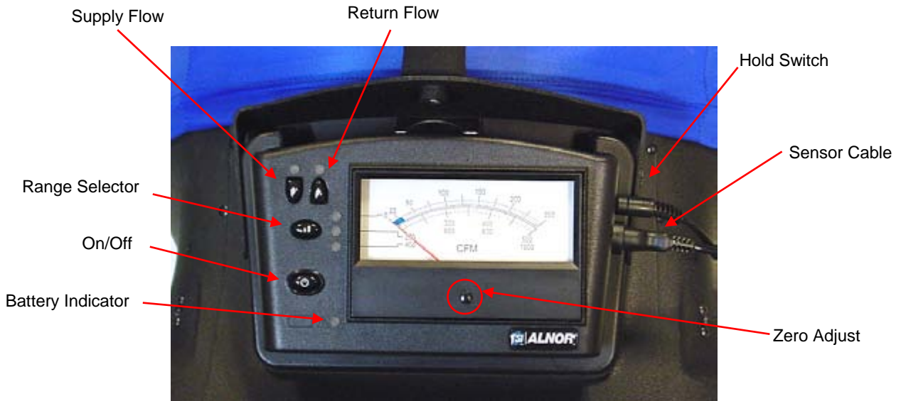
Figure 7 Analog Meter Components
