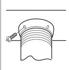
Note: Insert the M5 x 10 mm tripoint screw in the threaded pipe fitting as directed in the extension column instructions. If you are using an extension pipe without a notch, drill a 11/64 (0.172") dia. hole through the pipe and insert the screw through the pipe. Failure to do so could cause the assembly to fail.
