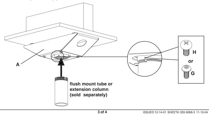
When attaching anti-vibration mount (**A**) to flush mount tube or extension column (both tube and column are sold separately ), tighten at least four complete turns ending with one of the small threaded holes aligned with slot in the end of flush mount tube or extension column. Insert and tighten one M5 screw (**H**) to lock tube position (shown below on right side). **Note: For security the M5 philips screw (H) can be replaced with M5 socket-pin screws (G).**
