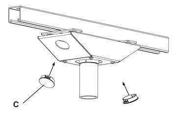
**OPTIONAL:** Place grommet (**F**) on anti-vibration mount (**A**) and place one finishing cap (**C**) on other end of anti-vibration mount (**A**). Route cords through extension column and out cord management holes in anti-vibration mount (**A**).
