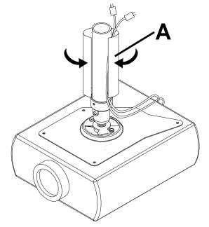
Make sure flaps from cord wrap (A) overlap each other. For finished look, turn cord wrap until the seam is facing away from view.
