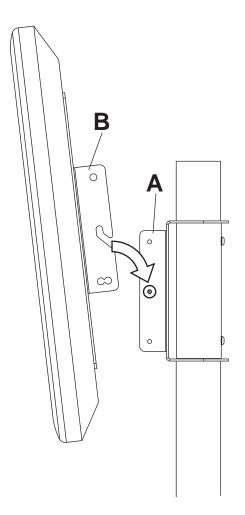
Insert two 1/4-20 x 12mm screws (**C**) into holes indicated below for desired display orientation. Adjust display then secure with two 1/4-20 x 12mm screws (**C**). Tighten all screws using 4mm allen wrench (**E**).
