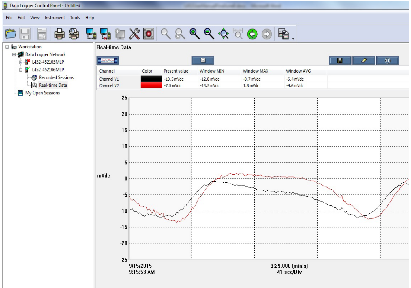
Figure 42. Data Logger Control Panel (instrument connected)
