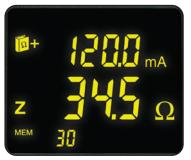
Displays the leakage current and loop impedance at the test frequency
