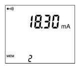
When the measurement has stabilized, you can press the **HOLD** key to freeze it and/or **MEM** to record it in memory. You can also use the AUTO-HOLD function (see §2.4) to freeze the measurement automatically when the clamp jaws are opened. This can be useful when you have only one hand free to make a measurement. To facilitate making measurements, you can configure an alarm on the current measurement value (see §2.4).
