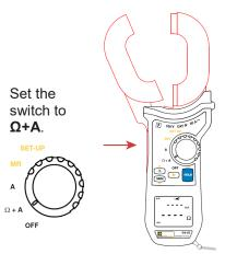
Press the trigger to open the jaws, and clamp around the conductor that is part of the ground system to be measured.
