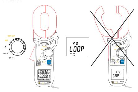
If the instrument fails to complete self-calibration, the error message **Err. CAL** is displayed. If this happens, turn the instrument OFF and ensure the air gaps are clean. Then turn the instrument ON.
