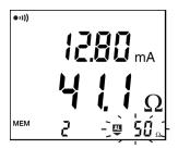
The alarm indicator on the display blinks and the instrument emits a continuous audible signal.
