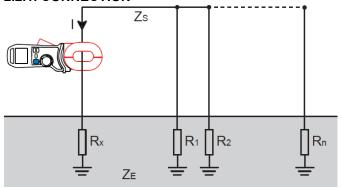
The ground electrode to be measured ( $R_X$ ) is in a series/parallel arrangement with other ground electrodes via the earth impedance ( $Z_E$ ) and physical connection to other resistance paths ( $Z_S$ ). The measured impedance will be slightly greater than  $R_X$  assuming the downstream impedance is very low. For example: If  $R_X$  is 21 $\Omega$  and  $Z_S/R_1-R_n$  is effectively 0.6 $\Omega$ , the Model 6418 will read 21.6 $\Omega$ .
