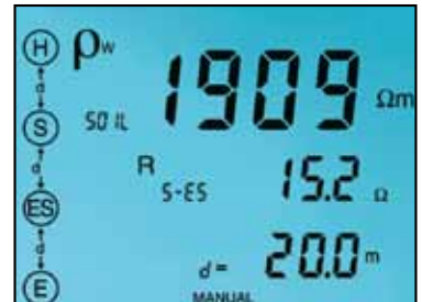
The Wenner test displays test lead connection, soil resistivity ( \rho ) test results, electrode spacing and resistance.
