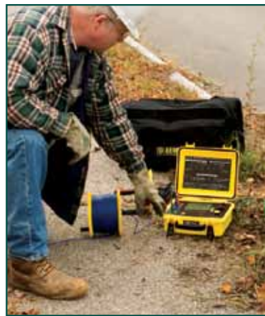
The Model 6470-B quickly checks ground rod resistance with its Connect – Press – Read approach.
