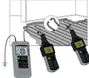
Fault detection in radiant heating systems
