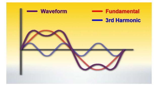
The combination of these two waves – the fundamental and the third harmonic – produces the distorted wave shown in our example. Adding additional harmonics results in further distortion in the waveform.
