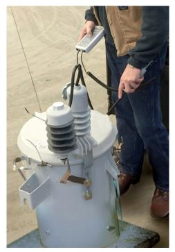
In each test, if the coil is functioning the green Transformer (T) PASS light blinks and the buzzer sounds. (Note that this center tap is sometimes switched in and out.)
