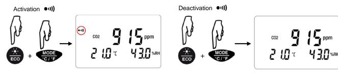
First press the **ECO** key, then, while keeping it pressed, press the **MODE** key.
