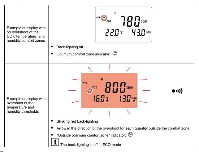
For the **1D** and **3D** modes, if the buzzer is active, it will sound intermittently upon the appearance of the  $\stackrel{oldsymbol{oldsymbol{B}}}{\odot}$  symbol.
