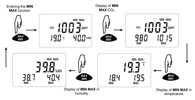
When the **MIN MAX** function is activated, recording of the minimum and of the maximum starts but the display of the three quantities measured makes it possible to continue using the device normally.
