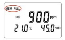
Any recording in progress is then stopped, and it is impossible to restart recording before emptying the memory.
