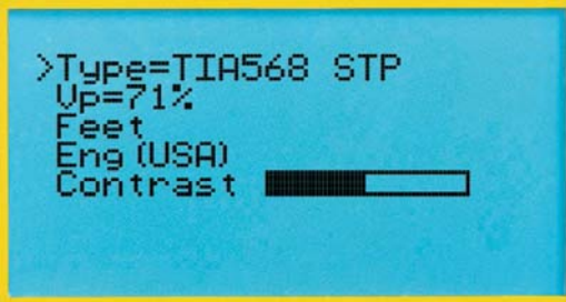
Quick and easy setup of cable type, Vp, feet/meter display, language and display contrast.
