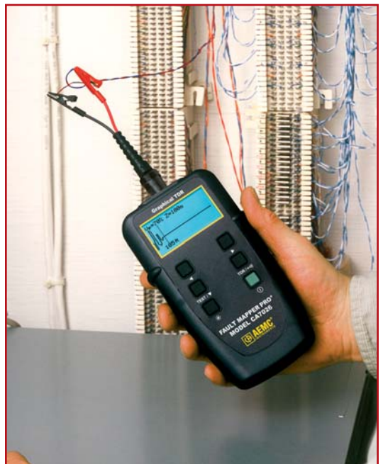
Model CA7026 testing cables in a telephone patch panel.
