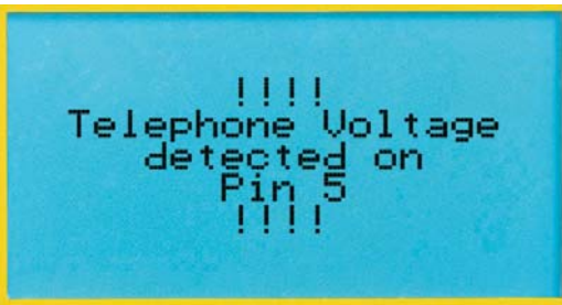
Automatic detection of live telephone voltage.
