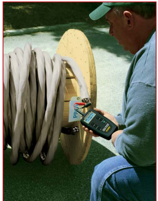
Model CA7024 is used to check length of a power cable on a reel.
