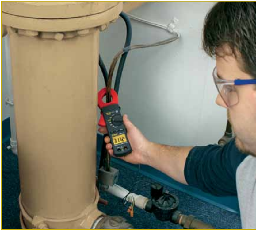
Measuring leakage current on a ground wire with the TRMS Leakage Current Meter Model 565
