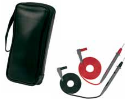
Model 565 includes two color-coded 5 ft test leads, batteries, soft carrying case and user manual.
