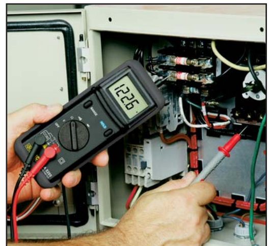
Model CA5205 measuring resistance in a relay cabinet.
