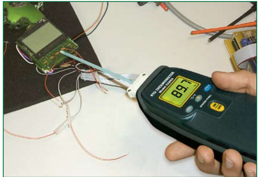
Precise RTD temperature sensor allows for accurate temperature measurement at specific points on the surface of electronic circuits.
