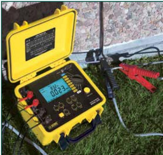
*Model 6250 conducting bond verification on a grounding system.*
