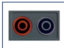
Jacks: Two standard safety banana jacks (4mm)
