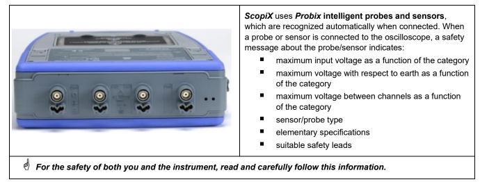
The trace color of the signal measured with a given accessory is set in the menu: "Green"  $\rightarrow$  "chX"  $\rightarrow$  "Probix". An interchangeable elastic or plastic ring is used to associate the color of the probe and the color of the trace. Scaling and units are configured automatically by the **Probix** system, allowing rapid measurements with no risk of error.
