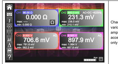
Channel 1 of the *ScopiX* is named CH1. It measures various physical quantities in addition to the signal amplitude measurements, using the appropriate *Probix* accessories. The other channels are voltmeter channels only (or current channels, when used with a *Probix* clamp).
