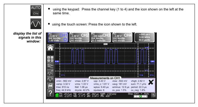
To start Auto measurements in the 4 channels:
